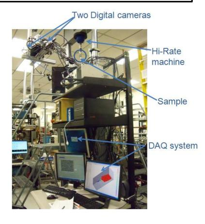
Custom Designed Hydraulic System Max Velocity=700 in/s (18.5 m/sec) over approx. 4 in (100 mm) Range
