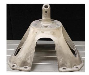
Current Wrangler Spare Tire Carrier (Thixomolded<sup>®</sup> AM60B)
