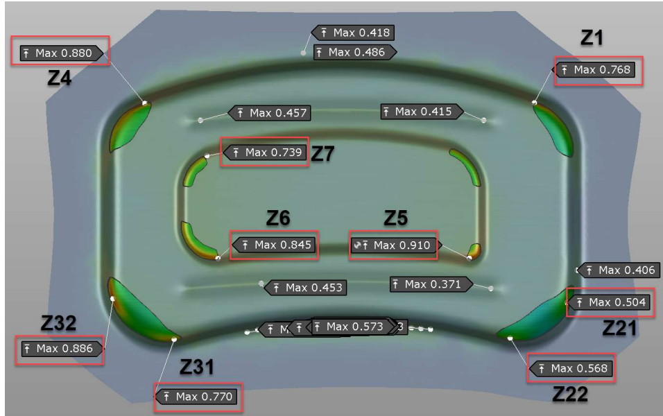
Figure 19 – Locations where max failure advanced criterion, an indicator of possible splits, was evaluated.
