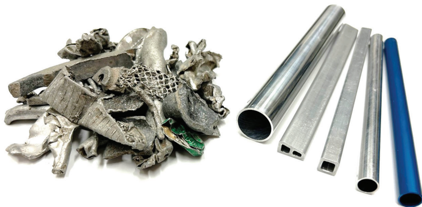
Fig. 2 — Left to right: Mixed Twitch Al alloy scrap supplied by Pacific Steel and Recycling; four Al alloy ShAPE-extruded tubes: a 1" diameter tube, a multicell extrusion, a square tube, a clear anodized tube; and a blue anodized tube made with Twitch scrap.
